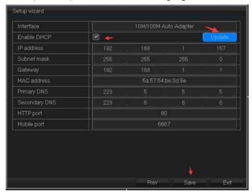
[DHCP Enable] Obtain IP address automatically.
