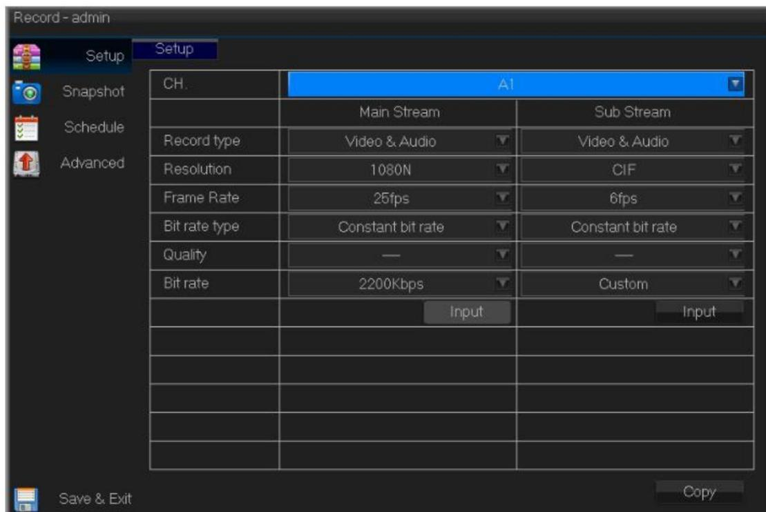
Main stream is used for local record, playback. Sub-stream is used for remote surveillance, such as: mobile surveillance. Dual stream technology can make playback and remote surveillance more smooth and clear.
